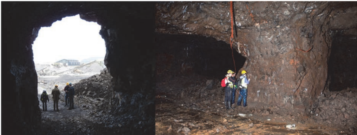
Figure 9.3: Abbeytown Mine; Left is adit entrance with quarry equipment in the background and right is underground pillar in the main index bed workings with Erris geologists taking samples.
