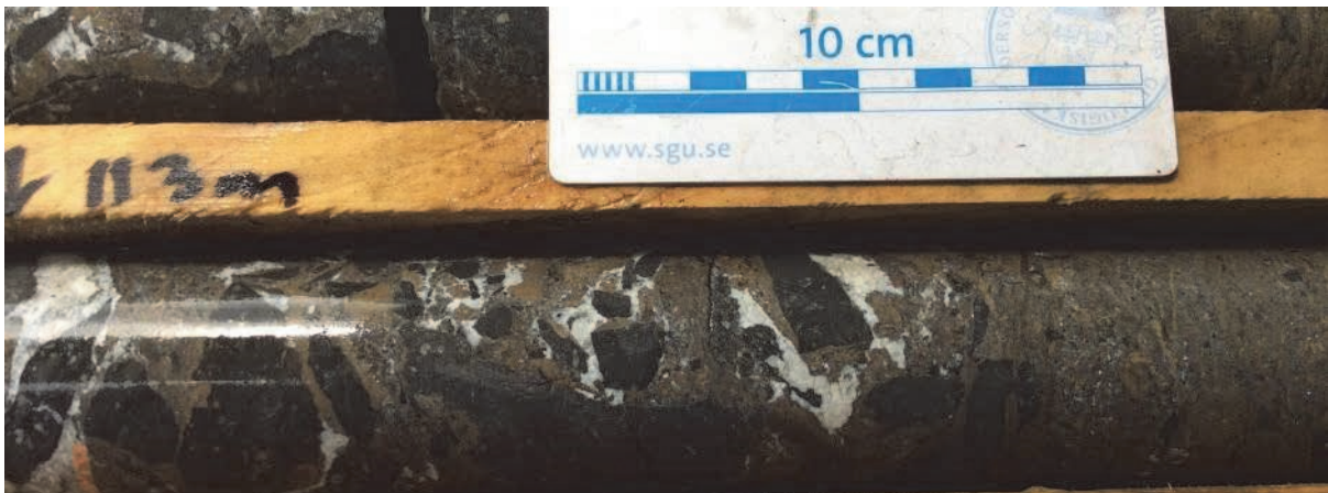
Figure 9.5: Strong sphalerite and galena mineralisation in karstic dissolution breccia in crinoidal limestone. This is typical style of mineralisation in the main zone from 110 - 121 m. Image is ER001 core at 113.0 m with 3.4% Pb, 9% Zn and 122 ppm Ag.
